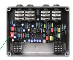
Internal Dip switches for E Booster allow you to fine-tune the boost frequencies and EQ settings. To hit your amp harde r while also adding some character to your tone And used the highest quality parts
